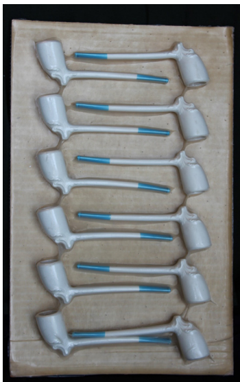
Figure 2: A dozen skin-packed pipes ready for shipping.
