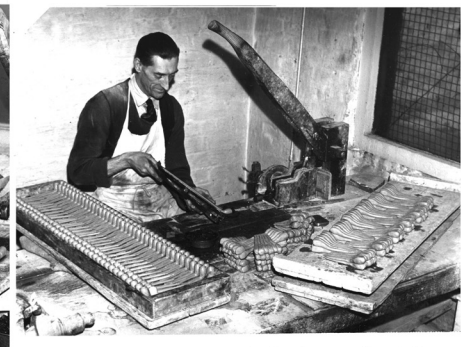
The rough "rolls" of clay seen in the tray on the right are moulded in a second into their final shape by John Hill, of Baguley, who has been doing the job for 26 years. The still moist pipes in the tray on the left are later taken to the drying room.
