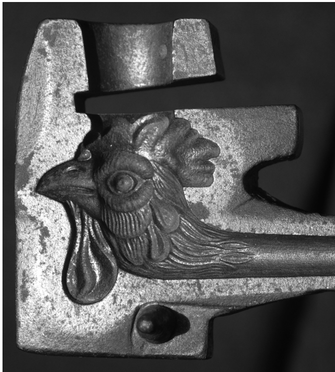
Figure 3: Mould detail showing the cockerel's head. There is a copper insert that has been used to form the bird's nostril (photograph by the author).
