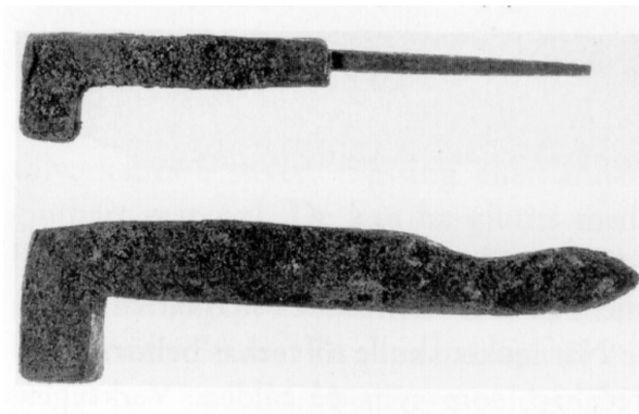
Figure 3: Anvils for the stem and bowl of the pipe respectively.
