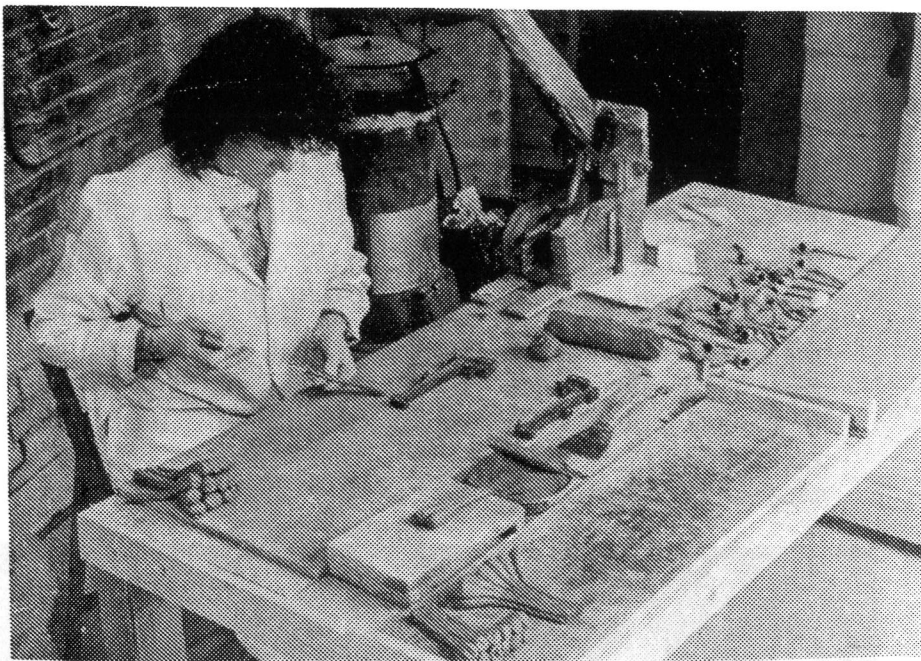
Fig. 8: Inserting the wire into the clay
